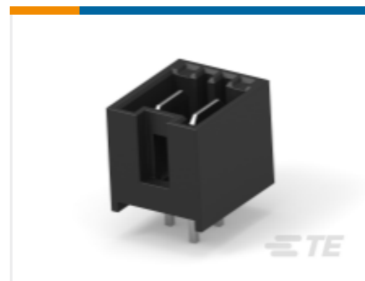
TE Part # 2232000-2 2P, RAST 5 Tab Header, THV,black, tin
